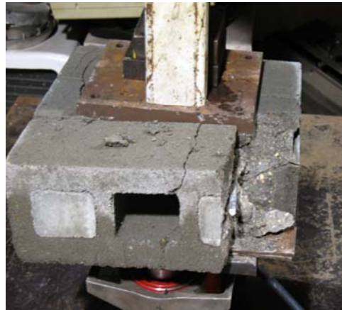
3/8" 2-cavity. Representative failure
