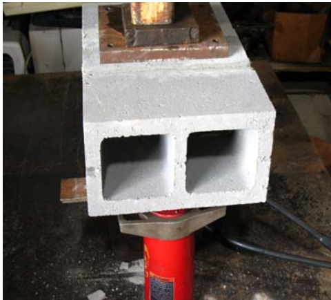
2-cavity mortar joint. Representative pre load
