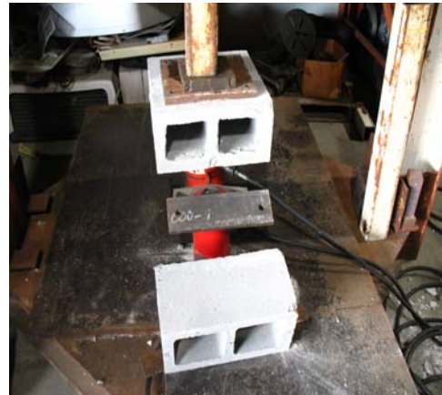
2-cavity mortar joint. Representative failure
