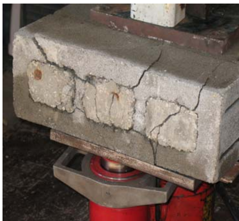
5/8" 3-cavity. Representative failure
