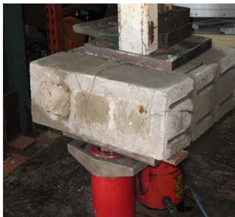
1/2" 3-cavity. Representative failure
