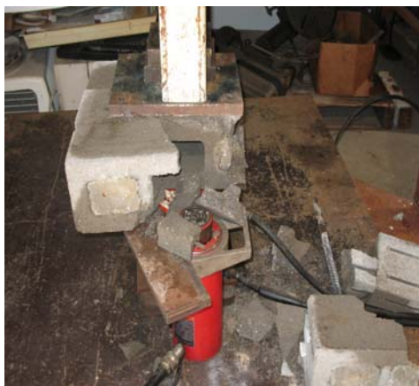
5/8" 2-cavity. Representative failure
