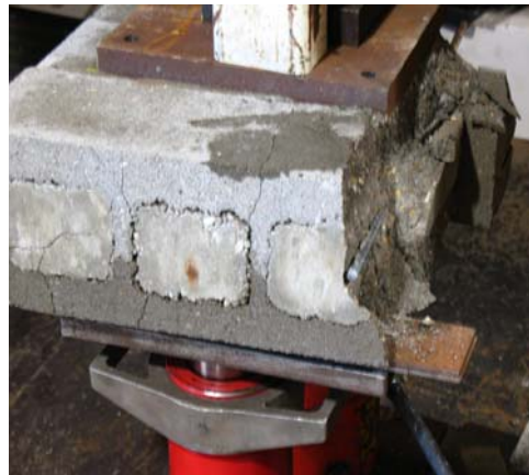
3/8" 3-cavity. Representative failure
