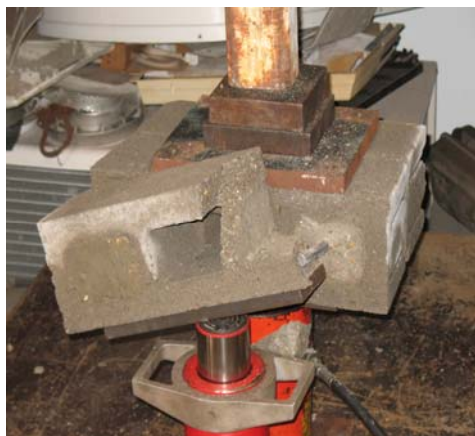
1/2" 2-cavity. Representative failure
